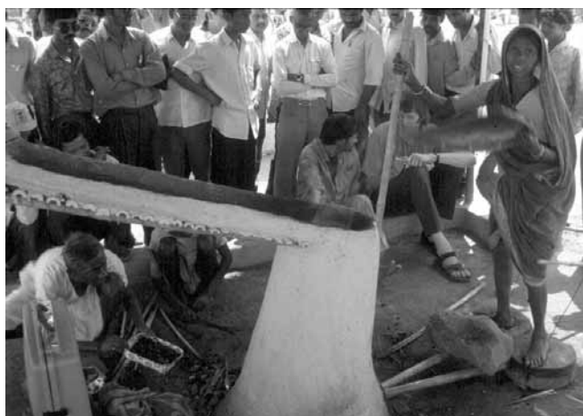
Figure 2. An iron smelting furnace at Bhilai, Madhya Pradesh, India in 1994. The husband is bottom left watching the slag tapping hole while his wife works the bellows. In the background can be seen various onlookers and the author taking notes.
