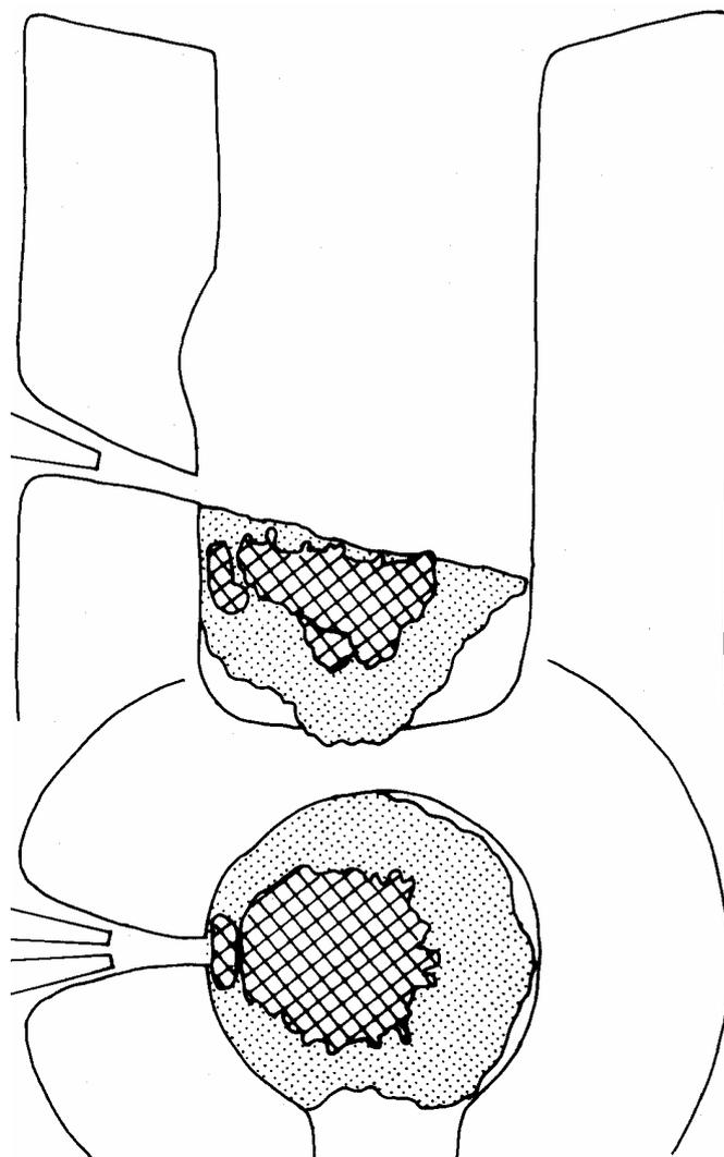
XP92 results, showing the location of the cast iron blocks (hatched) within an agglomeration of viscous low iron slags (stippled). Scale 1:10.
